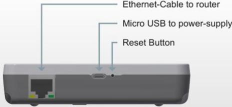
1. Make sure power is connected (Micro USB).
